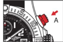
2. To interrupt the measurement, press pushpiece **A** once more. To restart the time measurement, press pushpiece **A**. This procedure makes it possible to add up several short times.
