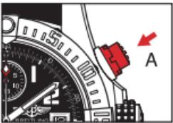
2. Stop the measurement by pressing pushpiece **A** once more. The measurement is made in hours [totalizer **1**], minutes [totalizer **2**], seconds and  $\frac{1}{4}$  of a second [hand **3**].
