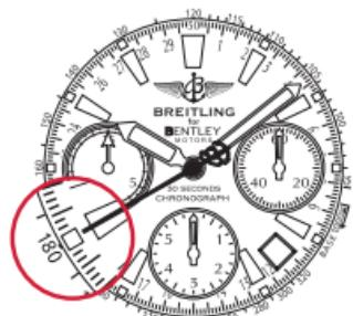
*Example 2:* If it takes 36 seconds to cover one kilometer or one mile, the average speed is 100 km/h or 100 mph respectively.
